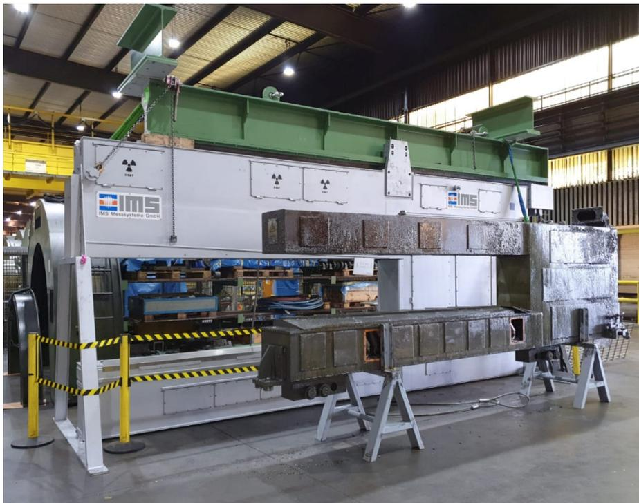
The material behaviour and mechanical dimensions of rolled aluminium must be constant over the complete length and width of strip within the tightest tolerances. Only in this way can the evermore exacting quality demands of downstream processors be satisfied. With the several thousand metres of strip material wound on to a coil involved, this is a challenge and requirement for manufacturers that can only be met by using measuring systems placed at significant points in the production process.
