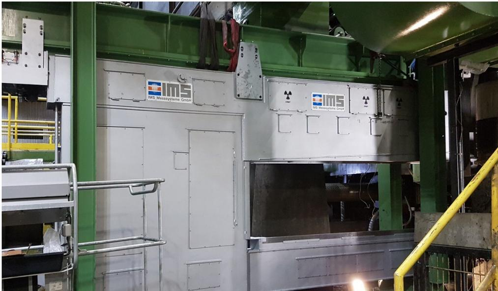
After just 10 months of operation, the customer has confirmed that measuring accuracy by the new IMS x-ray thickness profile measuring system has increased ten-fold compared to the former isotope measuring system. Thickness and thickness profile can now be controlled much more precisely. The exchange of the measuring systems has also optimised output, while simultaneously reducing the scrap rate, thereby minimising losses.
